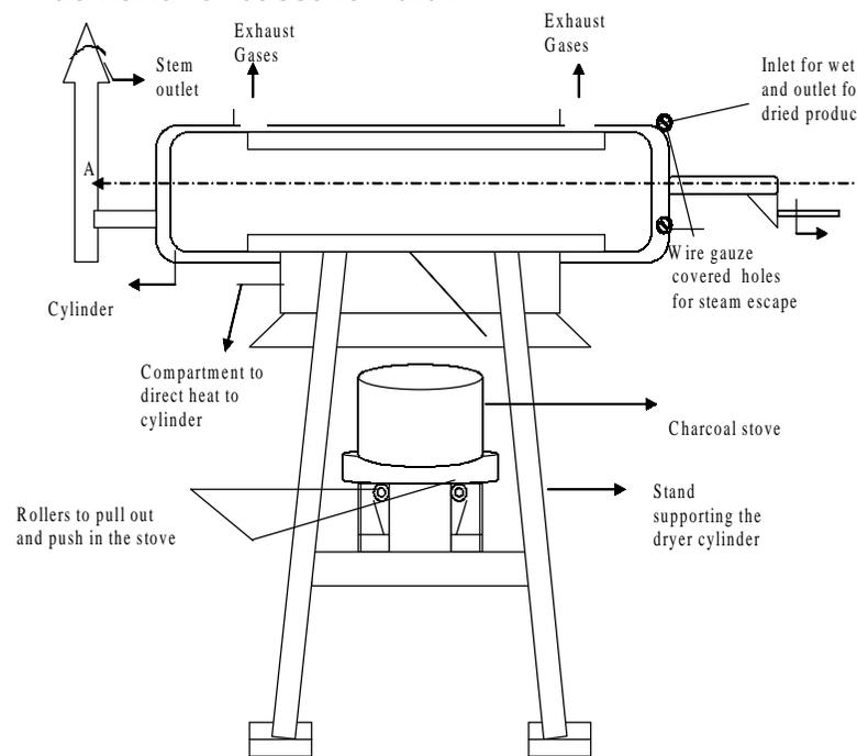
**Fig. 7: UNAAB Fufu Rotary Drier**
